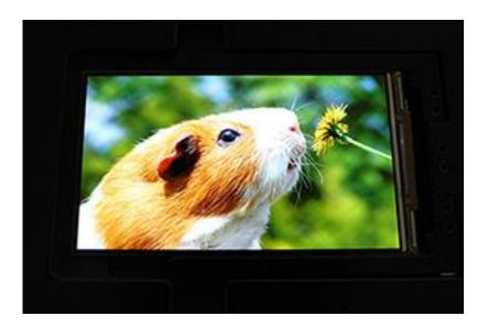
The new 5.5-inch TFT-HD with On-Cell Touch AMOLED display achieves high contrast and wide viewing angles while reducing display thickness.
